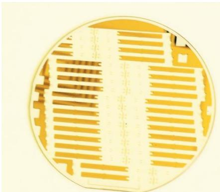
**Multifunctional integrated optical chip (MIOC)** is a monoblock hermetic product. It includes a linear polarizer, Y-junction coupler and two pairs of electro-optic phase modulators.
