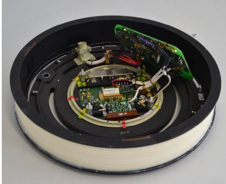
Figure 4. Internal arrangement of the SRS-5000 components in the device
