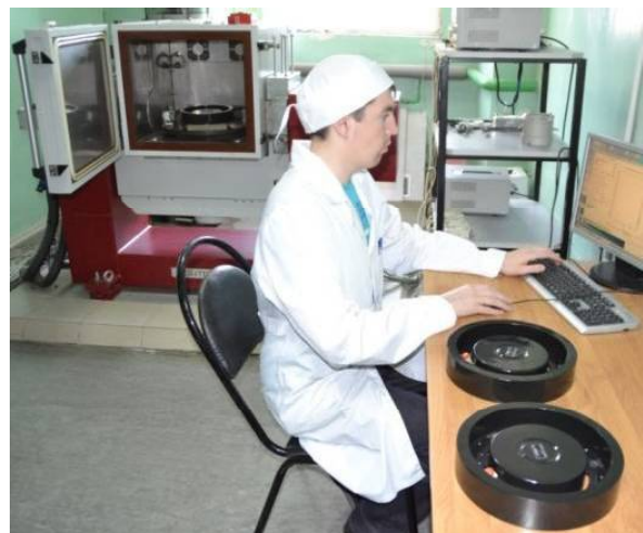
Figure 1b. Procedure of SRS-5000 devices testing in 2-axis motion simulator Acutronic AC2247-TCM
