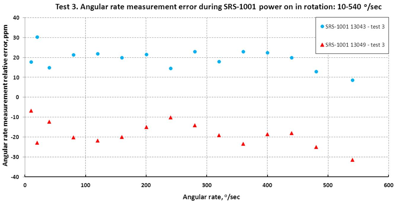
Fig. 8. SRS-1001 angular rate measurement error in tests with switching on in rotation
