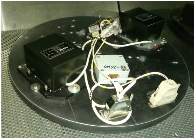
(a) IMUs with definite (-Z) axes along centripetal acceleration
