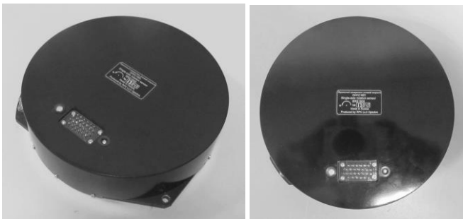
Fig. 12. Image of FOG SRS-1001 with extended dynamic range
