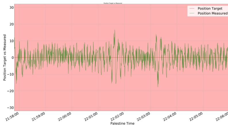
Figure 18: Azimuth position of the payload while in acquire mode (green line) with respect to our target (red line at  $0''$ ). An amplitude of  $15''$  is enough to center the target star into our science detectors using the tip/tilt mechanism.
