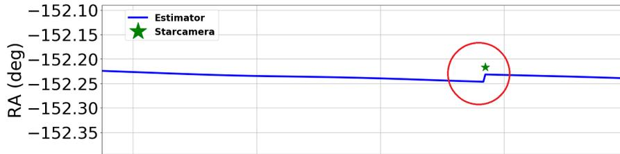
Figure 6: This zoomed in portion of the image shows that after a long period of time (over 20 minutes) without star camera solutions and just using the gyroscopes information, the RA of the estimator was only off by  $\sim 155.23^\circ - 155.225^\circ = 0.005^\circ$  or  $18''$ . Notice how the estimator (blue) corrects the position weighting in the latest star camera pointing solution.
