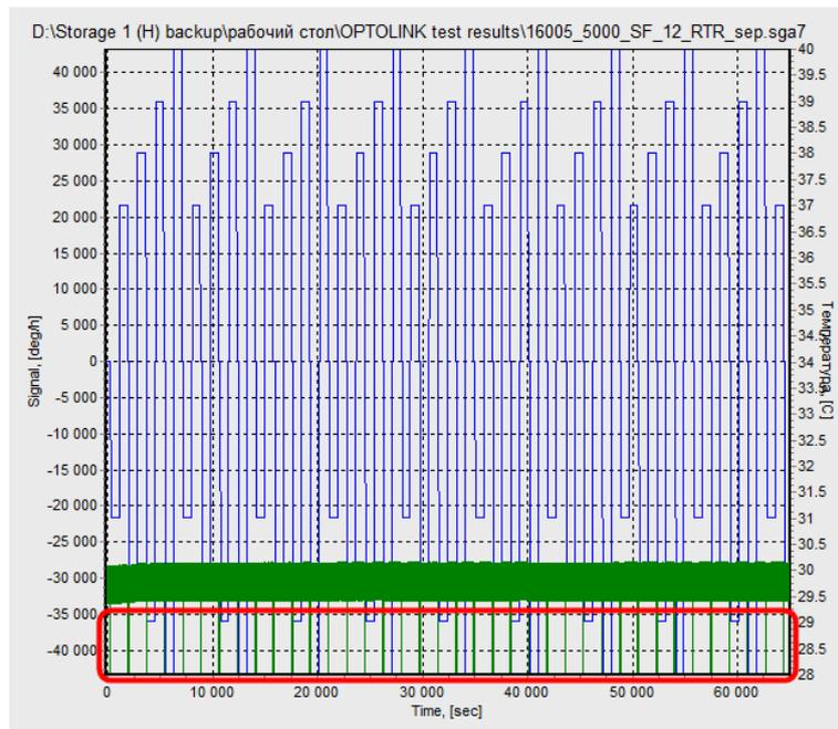
Figure 14. Scale factor run-to-run stability tests: raw data
